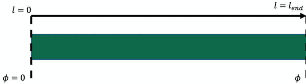
Figure 3.3: Constant cross-section dielectric rod. As a DRA, this rod radiates at the feed and terminal ends. According to the discontinuity radiation principle, fields from both the feed and terminal planes contribute to the far-field radiation pattern.
